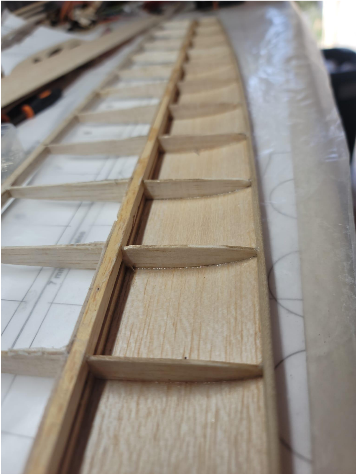
Top sheeting in place, now time the bottom
