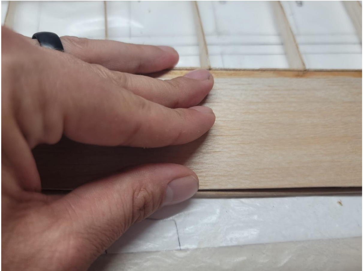
Double checking the fit once the sheeting is bend over the ribs.
