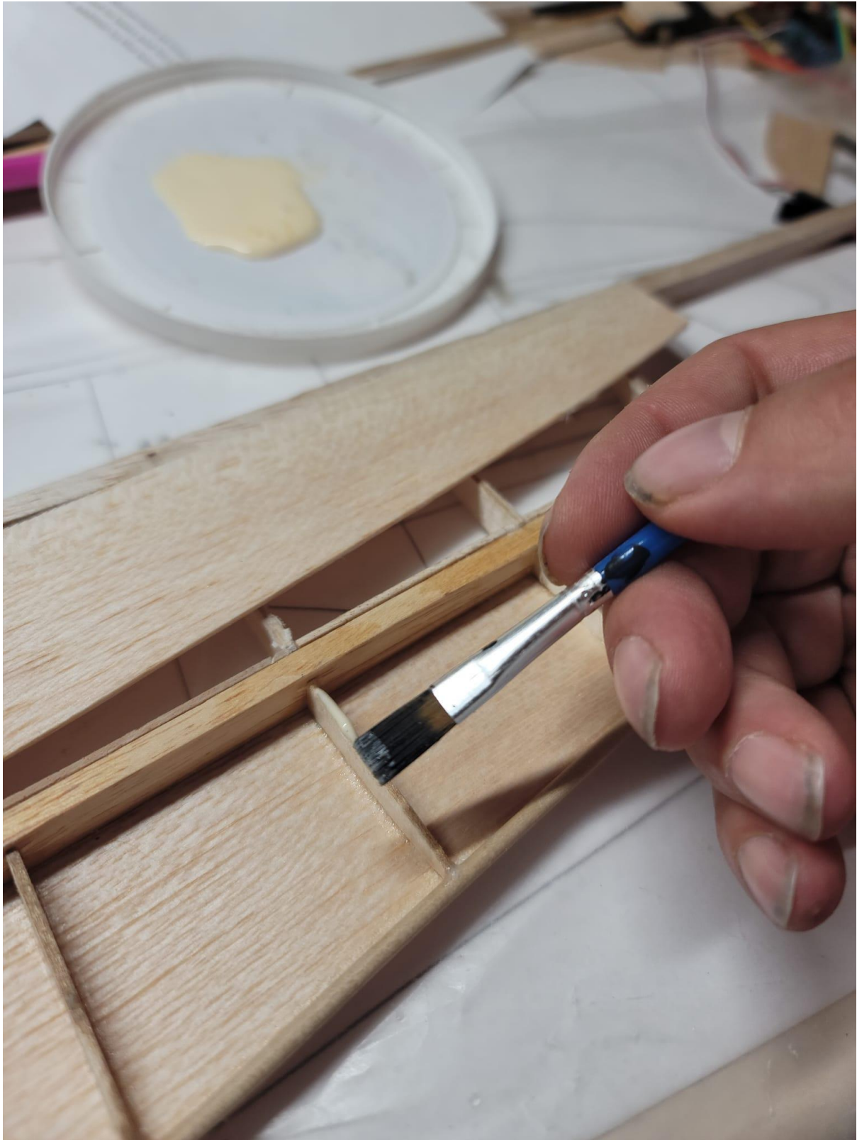
A touch of wood glue for the bottom ribs so we have some work time getting bottom sheeting in place.
